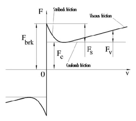
The Stribeck friction,  $F_S$ , is the negatively sloped characteristics taking place at low velocities (see [1]). The Coulomb friction,  $F_C$ , results in a
