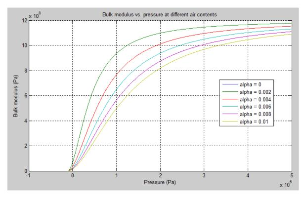
Cavitation is an inherently thermodynamic process, requiring consideration of multiple-phase fluids, heat transfers, etc., and as such cannot be accurately simulated with Simscape<sup>™</sup> software. But the simplified version implemented in the block is good enough to signal if pressure falls below dangerous level, and to prevent computation failure that normally occurs at negative pressures.
