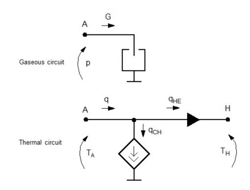
The diagram shows that the heat flow q to the chamber consists of two components:
