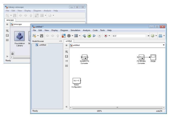
default solver set to ode23t, a Simulink-PS Converter block, and a PS-Simulink Converter block connected to a Scope block.
