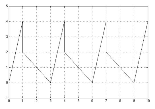
The signal starts at 0 and consists of two linear segments. The duration of the first segment is 1 second, the segment starts at 0 and ends at 4. The signal is discontinuous, and the end value of the first segment is different than the start value of the second segment, therefore they are connected by a vertical line. The second segment starts at 2, lasts for 2 seconds, and ends at 0, after which the sequence repeats.
