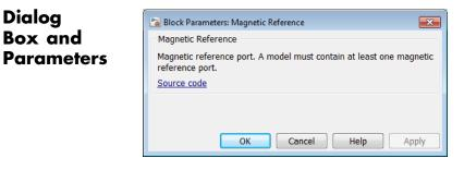
The Magnetic Reference block has no parameters.
