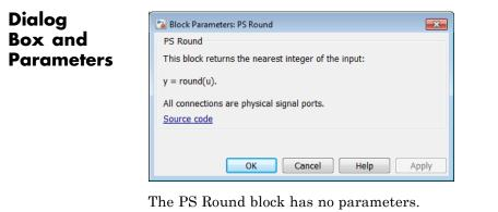
**Ports** The block has one physical signal input port and one physical signal output port.
