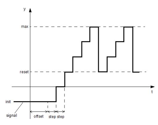
If the initial time offset is specified, the block outputs the initial signal value *init* until the simulation time reaches the *offset* value, at which
