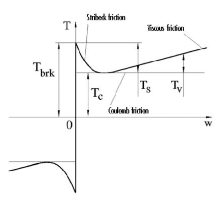
The Stribeck friction,  $T_S$ , is the negatively sloped characteristics taking place at low velocities (see [1]). The Coulomb friction,  $T_C$ , results in
