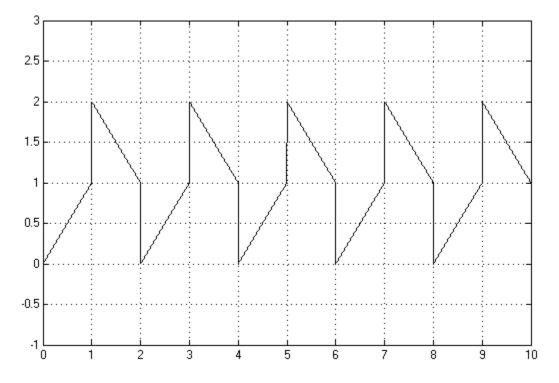
• Continuous — Each linear segment in the repeating sequence is defined by its duration and start value. The end value of a segment is the same as the start value of the next segment.
