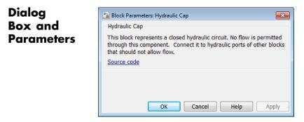
The Hydraulic Cap block has no parameters.
