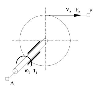
The wheel and the axle have the same axis, and the axis is assumed to be rigidly connected to the frame, thus making this mechanism an ideal converter of mechanical rotational into mechanical translational motion. The mechanism has two connections: a mechanical rotational port A, which corresponds to the axle, and a mechanical translational port P, which corresponds to the wheel periphery. The mechanism is described with the following equations:
