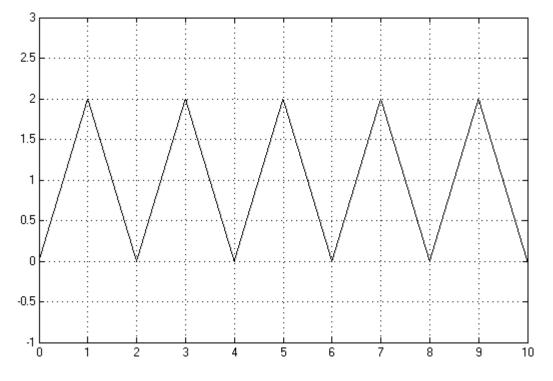
• Discrete — Each linear segment in the repeating sequence is defined by its duration and start value. The end value of a segment is the same as its start value.
