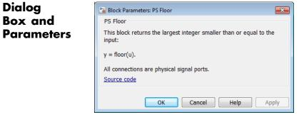
The PS Floor block has no parameters.
