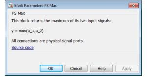
The PS Max block has no parameters.
